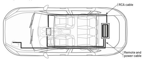
If you don't have any RCA outputs on your head unit you can use the high level input function.
