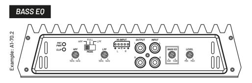
If everything is tuned correctly and the level/gain has been set, the BASS EQ should remain in default (0dB). This function will apply level/gain at 45Hz centre frequency. Be adviced that equing the bass from 0-12 dB is a lot, an increase of +3dB doubles the output! If used incorrectly, this can permanently damage your subwoofer.
