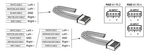
Use the right speaker cable for the job! Make sure to use the recommended size, and follow the polarity of the speaker wire from the speaker to the amplifier.
