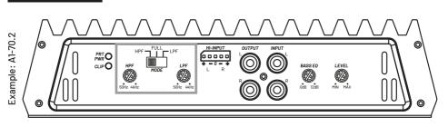
The crossovers are used to regulate the maximum and minimum frequencies each speaker is allowed to reproduce. The first thing you need to do is to find out the frequency response of each speaker you wish to connect to the amplifier. Don't allow the filters to pass through lower- or higher frequencies than your speakers can handle.
