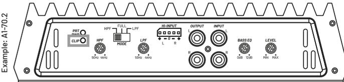
**CLIP.** When distortion exceeds 1%, the CLIP indicator glows orange.
