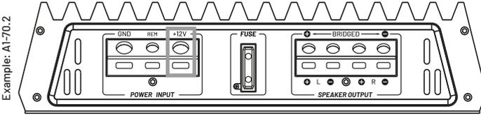
BATT +12V. Terminal input connection for +12V cable (+ power cable).
