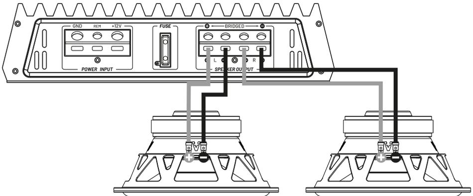
One bridged woofer (impedance minimum 4 Ohm):
