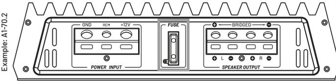
FUSE. Protects your amplifier from major damage in case of a power failure.
