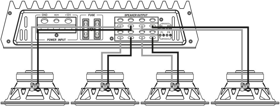
Two bridged woofers (impedance minimum 4 Ohm):
