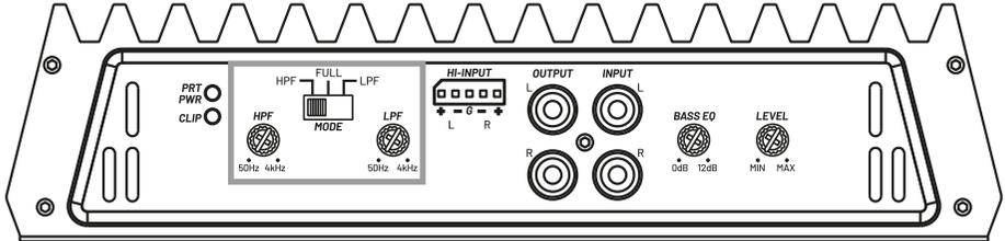
The crossovers are used to regulate the maximum and minimum frequencies each speaker is allowed to reproduce. The first thing you need to do is to find out the frequency response of each speaker you wish to connect to the amplifier. Don't allow the filters to pass through lower- or higher frequencies than your speakers can handle.
