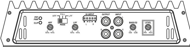
**LEVEL.** Sync your head unit's output signal with the amplifier.
