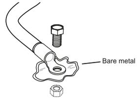
**Connect the power cable to the positive power source terminal,** preferably together with the vehicle +12V cable. A fuse holder needs to be placed on the cable at a 15-25 cm distance from the terminal and before any steel parts. **WARNING!** Install the fuses as the absolute final step when the rest of the installation is complete.
