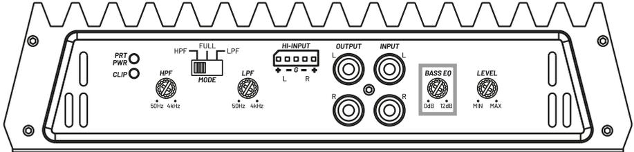
If everything is tuned correctly and the level/gain has been set, the BASS EQ should remain in default (0dB). This function will apply level/gain at 45Hz centre frequency. Be advised that equing the bass from 0-12 dB is a lot, an increase of +3dB doubles the output! If used incorrectly, this can permanently damage your subwoofer.
