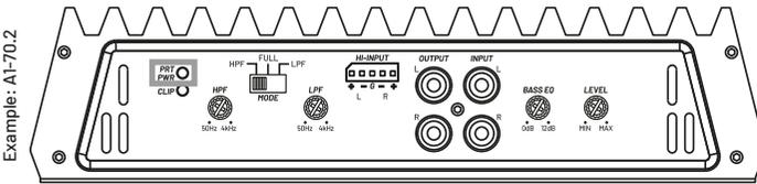
**POWER - PROTECT.** Power = Glows white when the amplifier is connected and on. Protect = Glows red when the amplifier indicates a failure.
