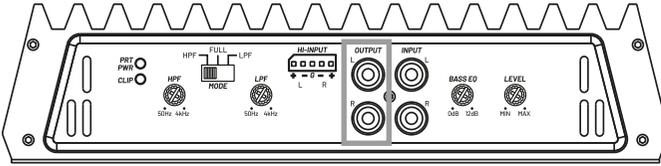
OUTPUT Left - Right. Send original signal to a second amplifier.
