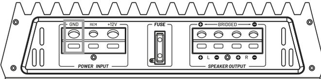
**GND.** Terminal input connector for ground cable (- power cable).
