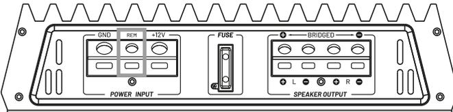
**REM.** Terminal input connector for the unit that controls the turn-on signal.
