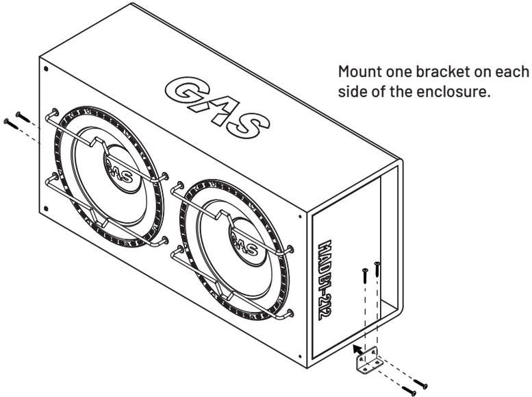
Mount one bracket on each side of the enclosure.
