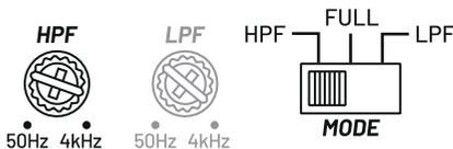
Set the high pass filter to 120Hz (PB1-46) or 100Hz (PB1-48) and the switch to HP/HPF mode. Compared to passive mode you can still change the level/gain between woofer and tweeter as you use different amplified channels. **WARNING!** Switch to FULL setting or lowering your high pass crossover point can damage your speakers and is not recommended.
