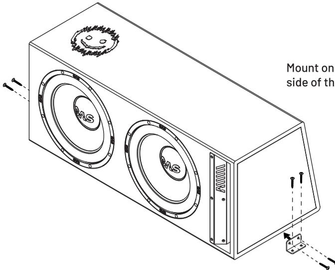
Mount one bracket on each side of the enclosure.
